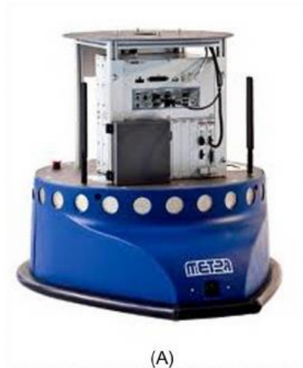
Figure 1.33 (A) SCITOS mobile general platform (SCITOS G5). (B) Robotic manipulator mounted on SCITOS G5.
