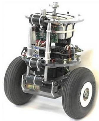
Figure 1.39 The NASA nBot (two-wheel balancing robot). Source: http://www.geology.smu.edu/~dpa-www/robot/nbot/nobot2/nb12.jpg .
