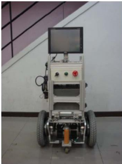
Figure 1.36 Mobile robot platform with spring-loaded castors for physical interaction with humans. Source: http://robot.kaist.ac.kr/paper/view.php?n=318 .
